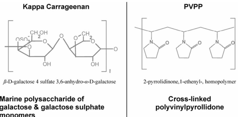
**Figure 7.** Combining polyvinylpyrrolidone (PVPP) with  $\kappa$ -carrageenan, Polyclar Brewbrite (International Specialty Products, Wayne, NJ) provides wort clarification and beer stabilization with a single addition to the kettle about 10 min before the end of boiling.
