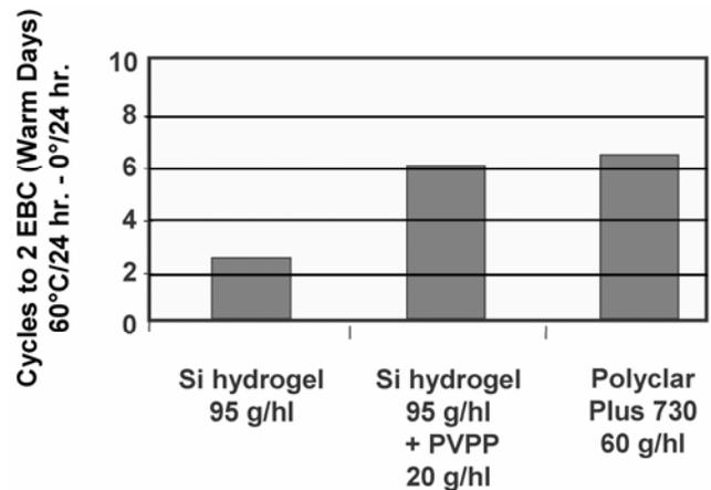
**Figure 15.** Predicted shelf life results—plant trial with Polyclar Plus 730 (composite 70% silica [si] plus 30% polyvinylpyrrolidone [PVPP]). In brewery trials, the admixture of PVPP and silica—Polyclar Plus 730—gave cost-effective efficacy of polyphenol and protein by a single addition to the beer stream without the need for specialized equipment. Balanced stabilization is efficient and cost effective.
