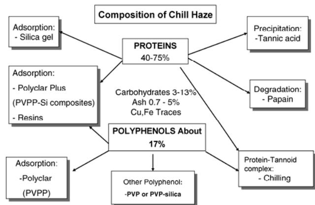
**Figure 6.** Options for colloidal stabilization of beer. The main stabilization options are highlighted in terms of their mechanistic actions. Some of the advantages and drawbacks of each are summarized in Table 2. Si = silica.
