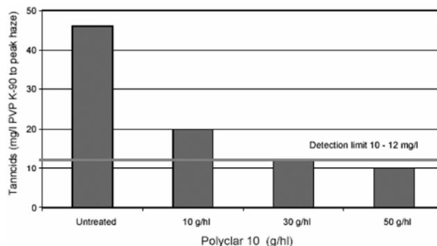
**Figure 13.** Tannoid reduction in an American lager treated with polyvinylpyrrolidone (PVPP). An addition of 10 g/hL resulted in a >50% reduction in the tannoid content of the beer. At 30 g/hL, the tannoid level was below the limit of detection of the assay.
