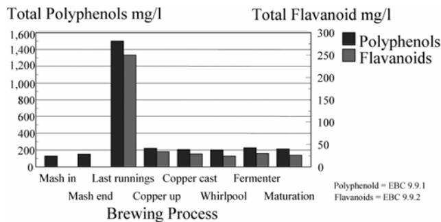
**Figure 5.** Change in polyphenols and flavanoids during brewing. In the brewhouse, avoiding the use of weak worts ( $<1.5^{\circ}\text{P}$ ) can play an important role in stabilization, since these contain very high levels of polyphenols.
