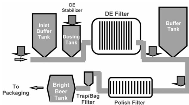
**Figure 12.** Schematic illustrating the possible addition points of the blended stabilizer. The highest efficacy is achieved by addition from a separate dosing tank to beer with low solids content. DE = diatomaceous earth.
