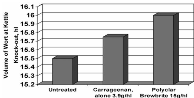
**Figure 8.** Increase in wort yield—commercial trial. Polyclar Brewbrite (International Specialty Products, Wayne, NJ) gave a 3.2% increase in wort yield as compared with that of untreated wort. A better solid-liquid phase separation in the whirlpool facilitates cold wort runoff, which can significantly improve process yield, without the necessity of trub recycling and its negative quality impact.
