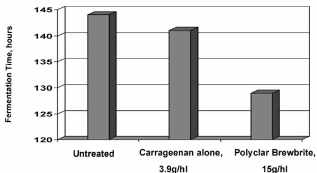
**Figure 9.** Decrease in fermentation time—commercial trial. Polyclar Brewbrite (International Specialty Products, Wayne, NJ) gave a 10% reduction in fermentation time as compared with that of the untreated control. The combination of carrageenan and polyvinylpyrrolidone (PVPP) may decrease the time to rack gravity, without impacting the overall attenuation or flavor profile of the beer.
