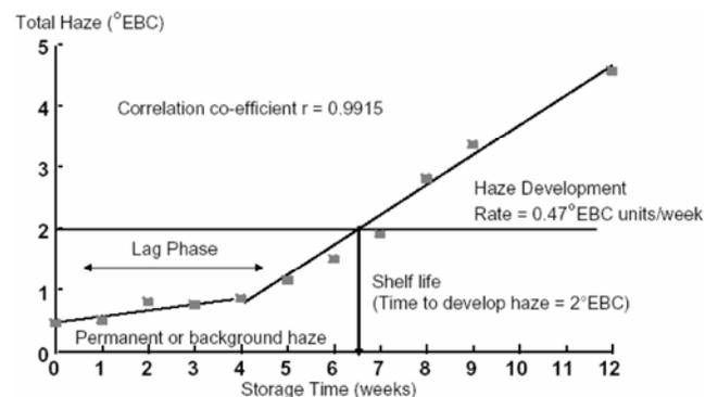
**Figure 4.** As the lower-molecular-weight polyphenols increase in size (polymerize), there is a significant increase in the rate of haze formation. This biphasic model of haze formation has been reported by many researchers. A well-stabilized beer is characterized by a long lag phase and a slow rate of haze development to the required shelf life of the beer.
